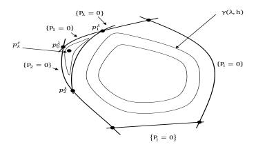
Assume that the system  $M_{\lambda} \frac{dH_{\lambda}}{H_{\lambda}}$  has a family of cycles  $\gamma(\lambda, h) \subset H_{\lambda}^{-1}(h)$  filling a connected component of  $\mathbb{R}^2 \setminus \{P_{\lambda}P_1 \cdots P_k = 0\}$ , which we denote by D. The period annulus D is bounded by  $\{P_{\lambda} = 0\}, \{P_1 = 0\}, \{P_2 = 0\}$  and some separatrices  $\{P_i = 0\}, i = 3, \dots, k$ .
