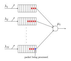
Fig. 2. Polling system associated with a given CPU core.
