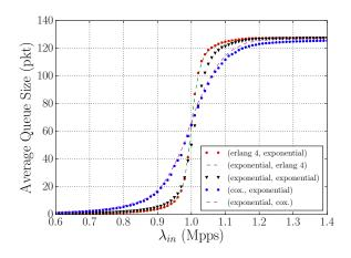
Fig. 6. Homogeneous CPU cores with N = 4 ports: Evolution of the average queue size  $\overline{q}_4$  when using different distributions of the packet inter-arrival time and packet processing time. Each data sample is associated with a couple of distributions (inter-arrival time distrib., packet processing time distrib.).
