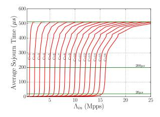
Fig. 10. Sizing the number of CPU cores in a virtual switch according the predicted average sojourn time.
