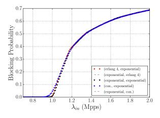
Fig. 7. Homogeneous CPU cores with N = 4 ports: Evolution of the blocking probability  $b_4$  when using different distributions of the packet inter-arrival time and packet processing time. Each data sample is associated with a couple of distributions (inter-arrival time distrib., packet processing time distrib.).
