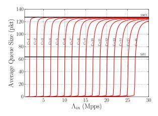
Fig. 11. Sizing the number of CPU cores in a virtual switch according the predicted mean queue size.
