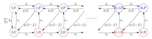
Fig. 4. Continuous-Time Markov Chain associated with queue *i*.
