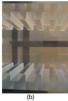
Figure 1 – Geometry of the corrugated channel. a) Schematic view, b) Photography of details of the face to face vertical corrugated plates.
