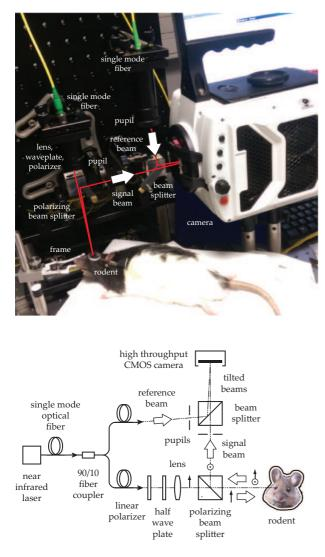
FIG. 1: Picture (top) and sketch (bottom) of the fibered Mach-Zehnder holographic interferometer used for retinal imaging. Off-axis interferograms of near-infrared radiation are recorded by the sensor array of a high speed camera.
