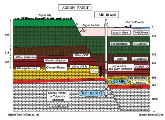
Figure 14. Schematic vertical cross-section, as established with the 1000 m deep AIG10 well (Cornet *et al.* 2004; Place *et al.* 2007). The figure outlines the two deep aquifers separated by the Aigion Fault (see the text).
