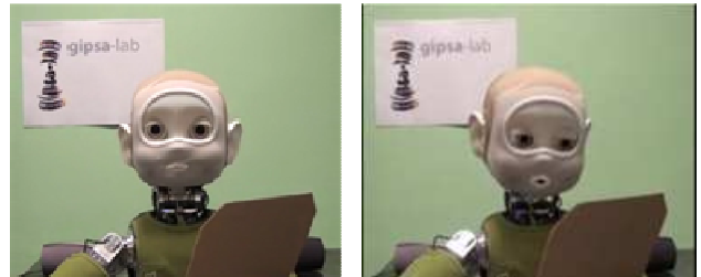
Figure 5. Robot’s gaze looking at subject’s face and scoring tablet.
