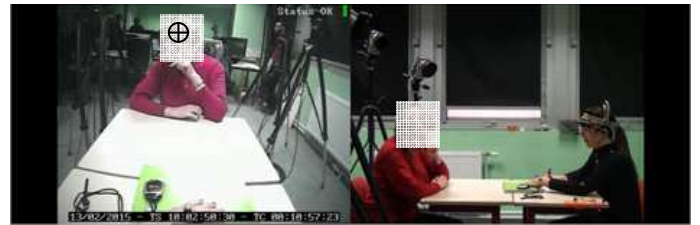
Figure 2. Visual data. Left: head-related view from the eyetracker scene camera. The marker superimposed to the scene camera features the current gaze fixation point. Right: side view from a fixed HD camera.
