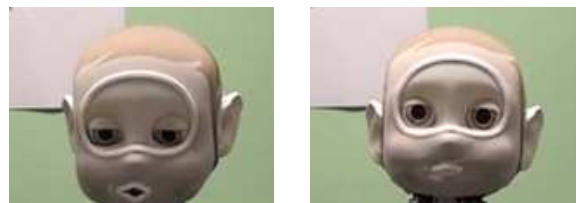
Figure 6. Robot’s eyelids with gaze looking down (left) or straight (right).
