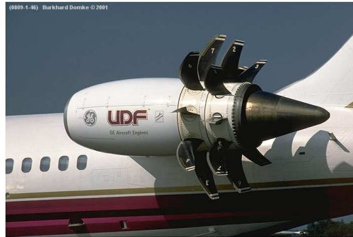
Figure 2: UDF ® de General Electric mounted on a McDonnell-Douglas MD-80.
