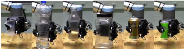
Fig. 2. Grasping deformable objects using gripper's built-in adaptive grasping mechanism.
