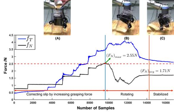
Fig. 6. Manipulating a deformable heavy jar by applying Algorithm 2. Plots show the recorded normal and tangential forces exerted by (here finger B) during the manipulation process.
