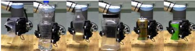
Fig. 2. Grasping deformable objects using gripper's built-in adaptive grasping mechanism.
