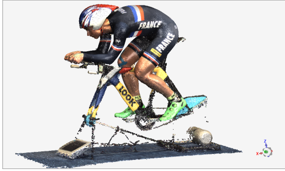
Figure 2: Model obtained with the Faro freestyle 3D.
