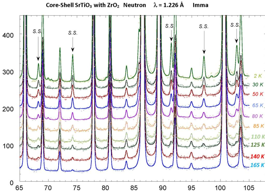
FIG. 8. Temperature evolution of enlarged part of Fig. 6 showing the evolution of superstructure peaks, as well as the calculated line from the  $Imma$  model up to the new (shifted) critical temperature.
