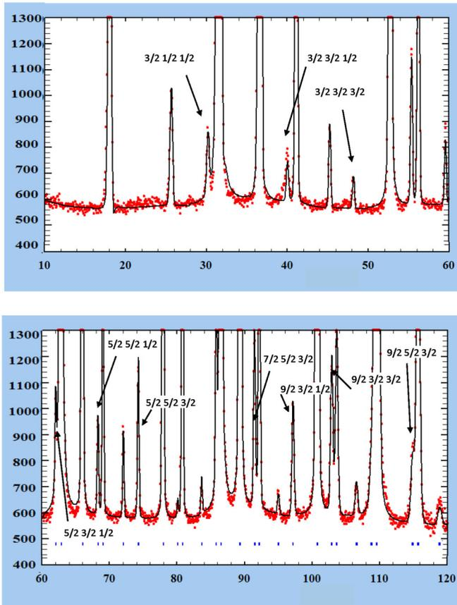
FIG. 7. Enlarged part of Fig. 6 showing all new (superstructure) peaks that appears during the transition in all types of samples, as well as the calculated line from the *Imma* model. The Miller indexes are given in the high temperature pseudocubic phase: They indicate that only antiphase rotations appears during the transition.
