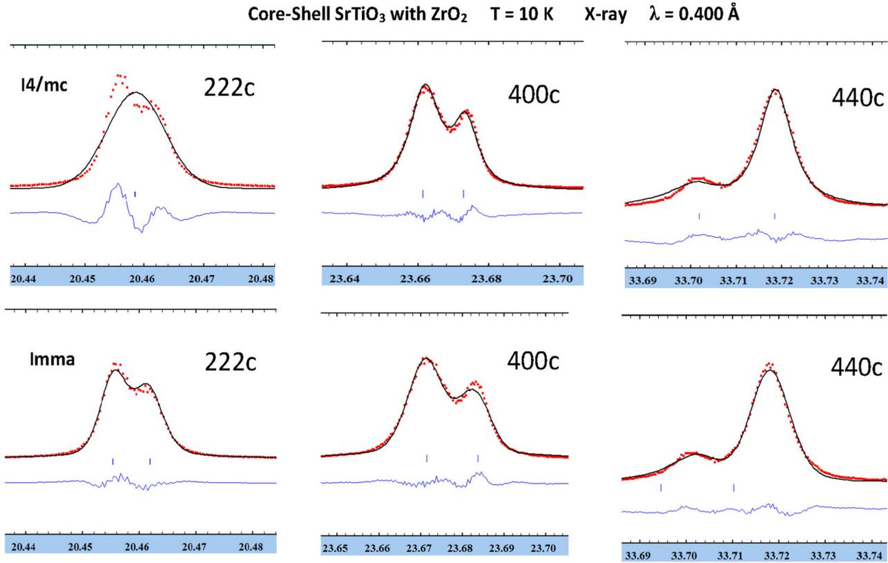
FIG. 3. The x-ray synchrotron selected Bragg peaks at 10 K of micrometric artificial CSS STO, with calculated lines and difference using the final structural *Imma* model (see below). It is clearly seen that 222c peaks cannot be explained by a tetragonal symmetry.
