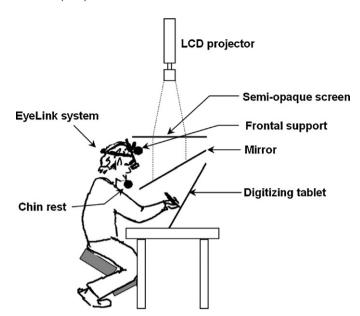
**Fig. 1.** Schematic representation of the experimental apparatus. Visual stimuli were projected onto a horizontal semi-opaque screen. Subjects faced an oblique mirror that reflected the images created on the semi-opaque screen. This setup created the illusion that visual targets were at the level of a third plane that corresponded to the surface of a large digitizing tablet.
