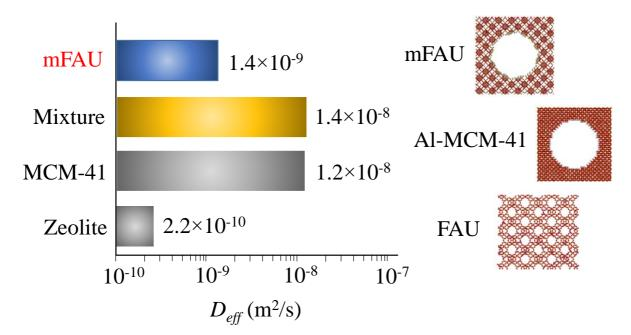
**Figure 3.** Effective diffusivity  $D_{eff}$  as determined from PFG NMR for hexane adsorbed at 298 K in FAU, Al-MCM-41, mFAU and a mechanical mixture of FAU+Al-MCM-41. For the mixture, the self-diffusivity corresponds to the fast contribution (Al-MCM-41). Note that the diffusivities  $D_{eff}$  are in a log scale for the sake of clarity.
