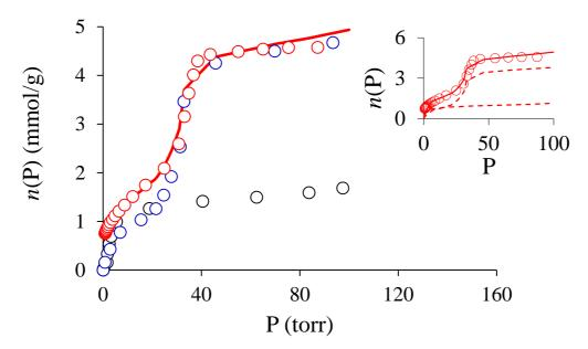
**Figure 1.** (color online) Hexane adsorption isotherm at 298 K in Faujasite zeolite (black ○), Al-MCM-41 (blue ○), and mesoporous FAU (red ○). The solid line is a fit of the adsorption isotherm for mesoporous FAU using the superimposition principle (*see text*). The inset shows the adsorption isotherm for mFAU (open circles) together with the linear combination (solid line). The dashed lines show the microporous and mesoporous contributions of the adsorption isotherm for mFAU.
