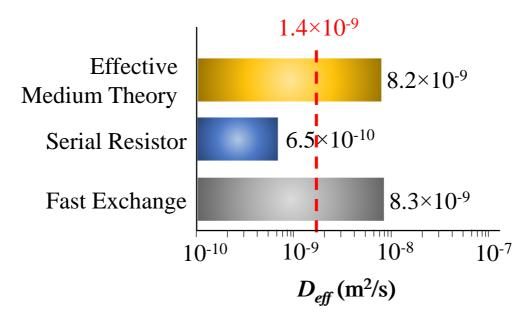
**Figure 4.** Predicted effective diffusivities  $D_{eff}$  for the different models considered in this work: fast exchange, serial resistor network, and effective medium theory. The dashed line indicates the experimental self-diffusivity of hexane in mFAU  $D_{eff}$  as obtained from PFG NMR. Note that the diffusivities  $D_{eff}$  are in a log scale for the sake of clarity.
