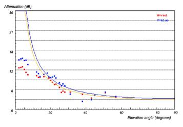
Fig. 12. Variation of foliage attenuation with the elevation angle for the first test site. Red color codes indicate H polarization and blue color ones V polarization.
