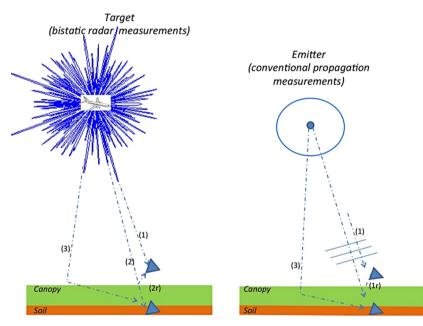
**Fig. 14.** Comparison of the two configurations: (right) conventional case where the emitter is a radar antenna located in the far field of the target; (left) bistatic and passive case where the plane body is used as a secondary emitter.
