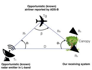
**Fig. 1.** The radar airport illuminates the planes, which in turn act as secondary sources. The signal coming from the plane is of unknown elliptic polarization. This signal is then collected by two receiving systems, but with the same receiving angle, because of the far-field condition: the first one, above the canopy, is the reference signal; the second one, below the canopy, is the signal attenuated by the forest.
