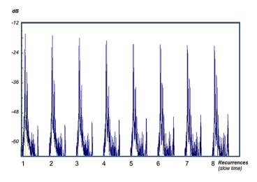
Fig. 9. Time signal emitted by the radar airport.
