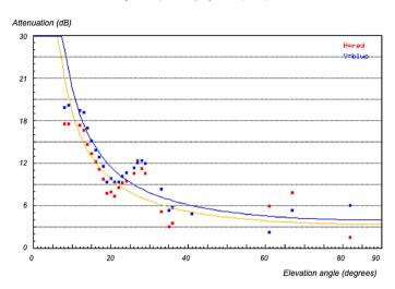
Fig. 13. Variation of foliage attenuation with the elevation angle for the second test site. Red color codes indicate H polarization and blue color codes V polarization.
