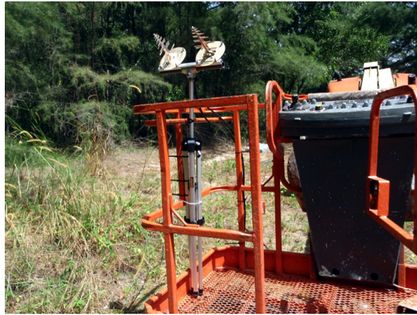
Fig. 8. Each receiving system—above and below the canopy—is comprised of two antennas: one vertically polarized, the other one horizontally polarized. The signal coming from the plane if of unknown polarization. When it is collected by the receiving systems, the antennas act like filters, so that one can determine the attenuation for the two copolarizations.
