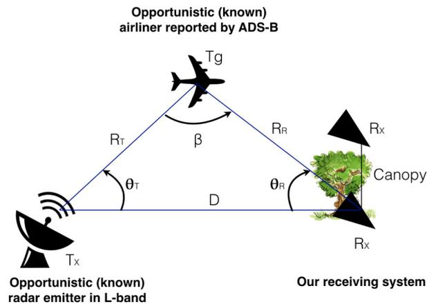
**Fig. 1.** The radar airport illuminates the planes, which in turn act as secondary sources. The signal coming from the plane is of unknown elliptic polarization. This signal is then collected by two receiving systems, but with the same receiving angle, because of the far-field condition: the first one, above the canopy, is the reference signal; the second one, below the canopy, is the signal attenuated by the forest.
