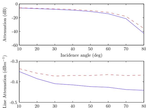
**Fig. 20.** Variation with the incidence angle of the total (top) and line (bottom) attenuation simulated over a mangroves-type forest in VV polarization (solid blue line) and in VH-polarization (dashed red line).
