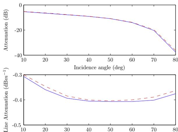
**Fig. 19.** Variation with the incidence angle of the total (top) and line (bottom) attenuation simulated over a pine-tree forest in VV polarization (solid blue line) and in HH-polarization (dashed red line).
