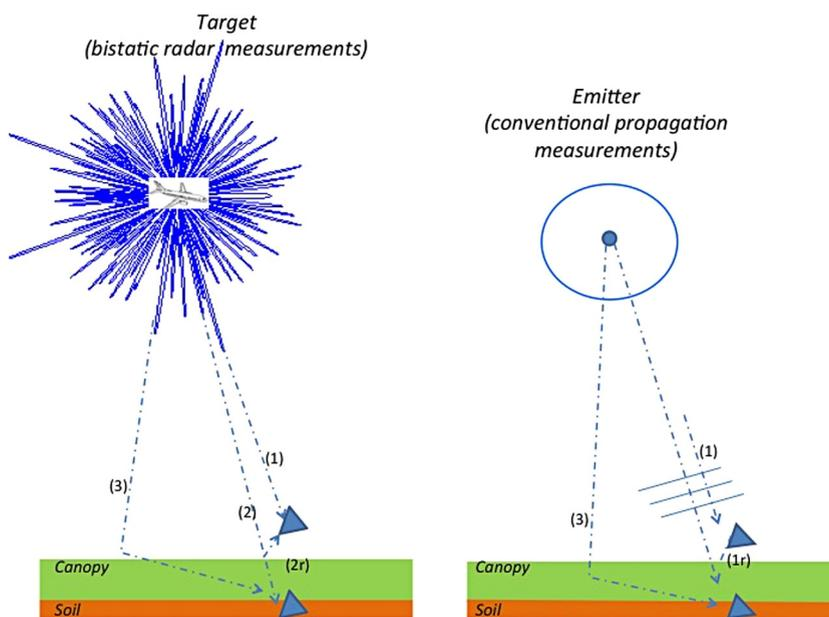
**Fig. 14.** Comparison of the two configurations: (right) conventional case where the emitter is a radar antenna located in the far field of the target; (left) bistatic and passive case where the plane body is used as a secondary emitter.
