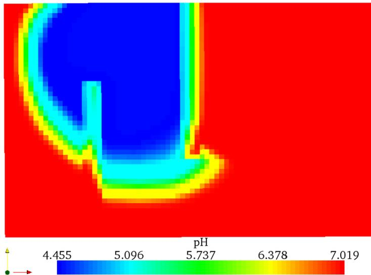
Figure 7.2: pH of the SHPCO2 test case at  $t = 95.13$  years (end of the first time-window for the domain decomposition simulation). The low pH-value can be seen as an indicator of highly-chemically reactive zones.
