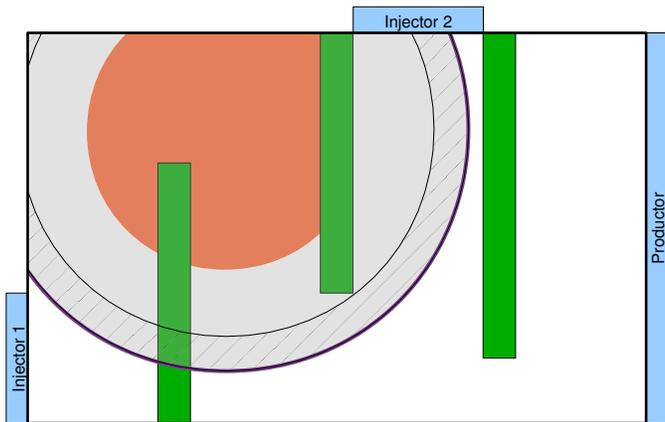
Figure 7.1: Choice of subdomains in the SHPCO2 2D test case. Orange: position of the initially present  $\text{CO}_2$ . Green: Areas with low porosity. Shaded grey: reactive subdomain. Violet solid line: Interface of the reactive subdomain. Hatched annulus: overlapping region between reactive and non reactive subdomain.
