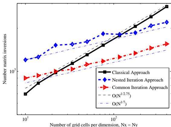
Figure 6.6: Number of matrix inversions versus number of discrete points per dimension ( $N_x = N_y$ ) for the classical approach (fixed point on the nonlinear interface problem), Nested Iteration Approach and Common Iteration Approach
