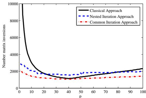
Figure 6.5: Number of matrix inversions versus parameter  $p$  of the Robin transmission conditions for the classical approach (fixed point on the nonlinear interface problem), Nested Iteration Approach and Common Iteration Approach
