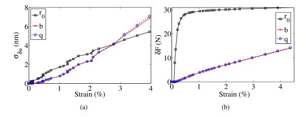
Figure 13: Root mean square value of the field  $\delta u_c$  (a) and sensitivity of the load calculated by homogenization (b) corresponding to a 20 % variation of each of the parameters  $r_0$ , b and q as functions of the mean strain
