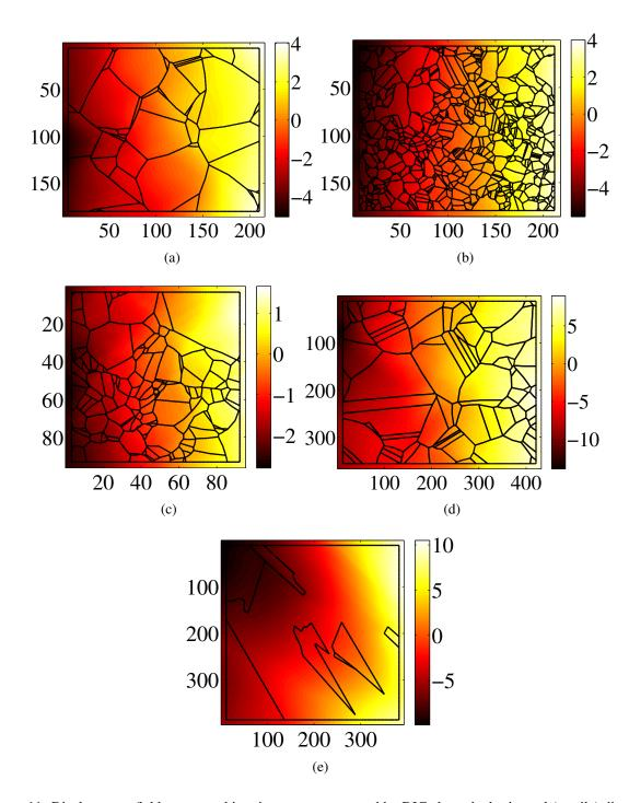
Figure 11: Displacement fields expressed in micrometers measured by DIC along the horizontal (tensile) direction for a mean tensile strain of 4 %, for the microstructures denoted  $A_{70}$  (a),  $B_{10}$  (b),  $C_{10}$  (c),  $D_{50}$  (d) and  $E_{1000+}$  (e). The microstructure boundaries are shown as black lines on these fields
