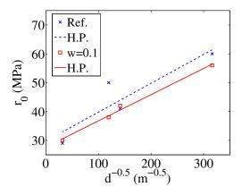
Figure 18: Identification of the Hall-Petch (H.P.) law from the values of the initial critical resolved shear stress  $r_0$  (dots) identified by homogenization and from the ones identified when w = 0.1
