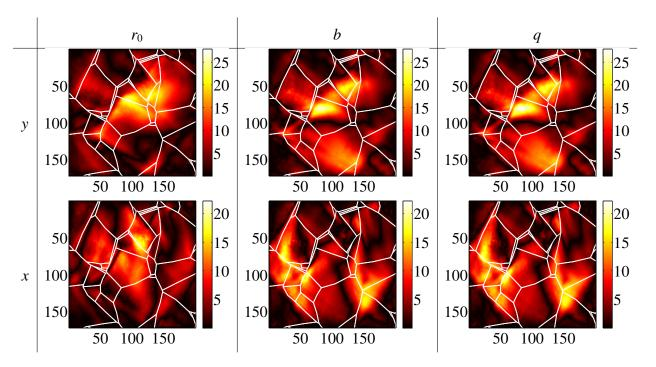
Figure 12: Absolute value of the sensitivity of the simulated displacement field  $|\delta u_c|$  (expressed in nanometers), for a 20 % (forward) variation of each of the parameters  $r_0$ , b and q shown along the horizontal y and vertical x directions for a mean strain of about 4 %. The spatial axes are expressed in micrometers
