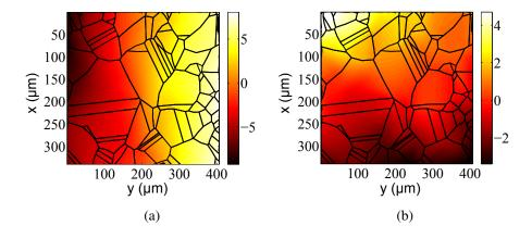
Figure 1: Displacement fields expressed in micrometers along the horizontal y (a) and the vertical x (b) axes simulated with the 2D assumption for a macroscopic strain of about 5 %
