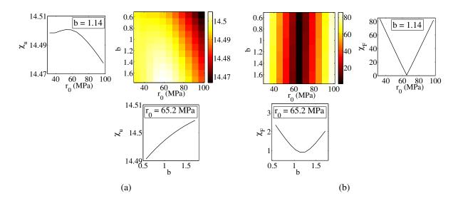
Figure 8: Cost functions  $\chi_u$  (a) and  $\chi_F$  (b) versus the values of the parameters  $r_0$  and b when the reference values are  $r_0 = 67$  MPa and b = 1.2
