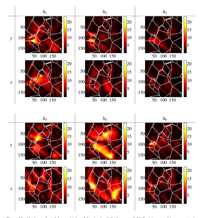
Figure 19: Absolute value of the sensitivity of the simulated displacement field  $|\delta u_c|$  (expressed in nanometers), for a 20 % (forward) variation of each of the coefficients of the interaction matrix shown along the horizontal y and vertical x directions for a mean strain of about 4 %. The spatial axes are expressed in micrometers
