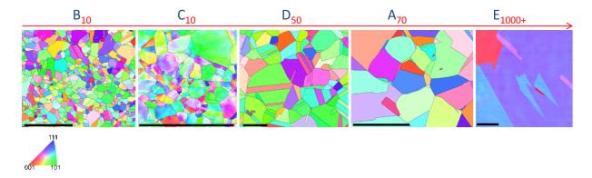
Figure 9: IPF of the the five studied microstructures sorted in increasing mean grain size order. The scale bar is 100 µm long
