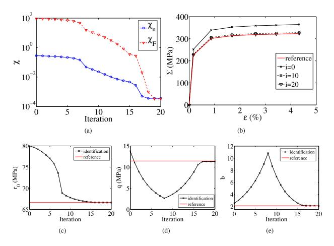
Figure 5: Cost functions  $\chi_u$  and  $\chi_F$  (a), macroscopic stress-strain curve (b) and parameters  $r_0$  (c), q (d) and b (e), as functions of the iterations i of the identification procedure performed with w = 0.5
