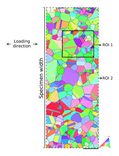
Figure 3: IPF and grain boundary maps of the full width of specimen  $D_{50}$ . The edges of the regions of interest denoted ROI 1 and ROI 2 are drawn with solid and dashed lines, respectively. The scale bar is 200  $\mu$ m long, and the specimen width (vertical in the figure) is 2 mm
