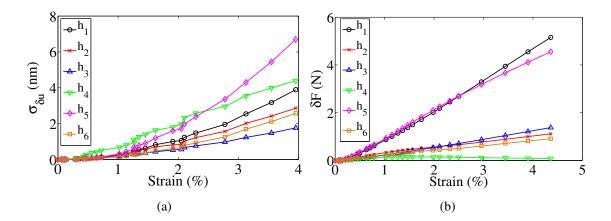
Figure 20: Root mean square value of the field  $\delta u_c$  (a) and sensitivity of the load calculated by homogenization (b) corresponding to a 20 % (forward) variation of each of the coefficients of the interaction matrix as functions of the mean strain
