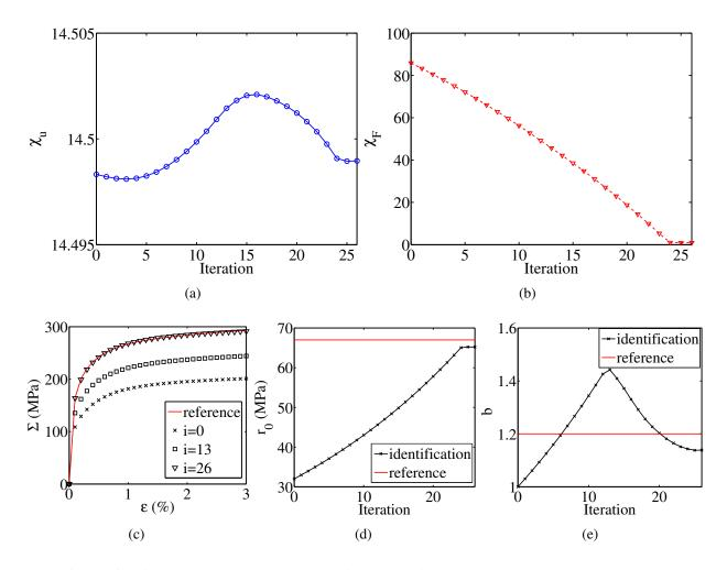
Figure 6: Cost functions  $\chi_u$  (a) and  $\chi_F$  (b), macroscopic stress-strain curve (c) and parameters  $r_0$  (d) and b (e), as functions of the iterations i of the identification procedure performed with w = 0.5
