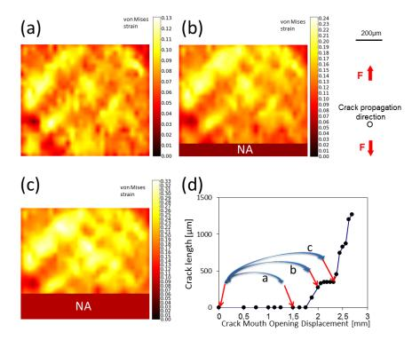
Figure 7: 2D sections of *cumulated* equivalent von Mises strain fields. (a) Direct correlation from CMOD = 0.0 mm to CMOD = 1.5 mm. (b) One cumulation from CMOD = 0.0 mm to CMOD = 0.0 mm. (c) Two cumulations from CMOD = 0.0 mm to CMOD = 0.0 mm to
