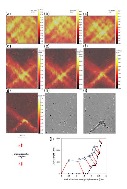
Figure 6: Overlay of incremental equivalent strain fields (half transparent) over the microstructure 1080  $\mu$ m ahead of the notch root. (a)-(g) 2D sections of laminography data and equivalent strain fields. The microstructure is shown in state n for incremental correlations between n and n+i. Two reference voids are encircled in white on the microstructure for every load step; (h),(i) microstructure showing damage and the final crack path; (j) load steps corresponding to the shown sections
