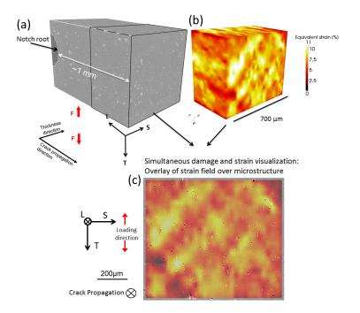
Figure 5: (a) 3D rendering of the initial microstructure and the ROI. (b) 3D rendering of the equivalent strain field in the extracted volume when CMOD = 1.5 mm. (c) 2D overlay of strain field over the initial microstructure
