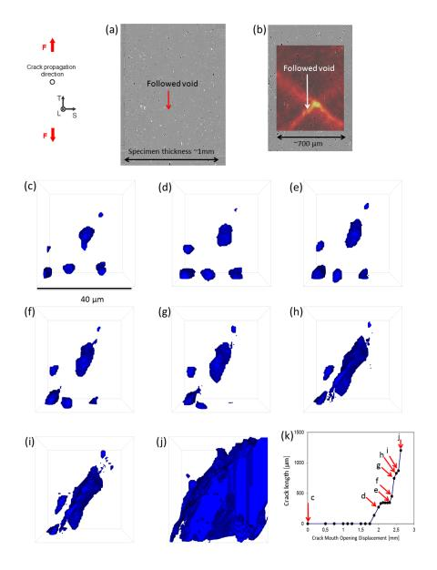
Figure 13: 3D void visualization of reconstructed laminography data. (a) Through-thickness section with location of the void 1125  $\mu m$  from the notch. (b) Overlay of strain field for step CMOD = 2.5 mm to CMOD = 2.563 mm over microstructure at CMOD = 2.5 mm. (c)-(j) Void growth. (k) Indication of the corresponding load step
