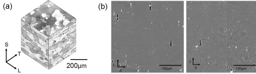
Figure 1: (a) Pseudo 3D cube showing the grain shapes (optical microscopy after etching).
