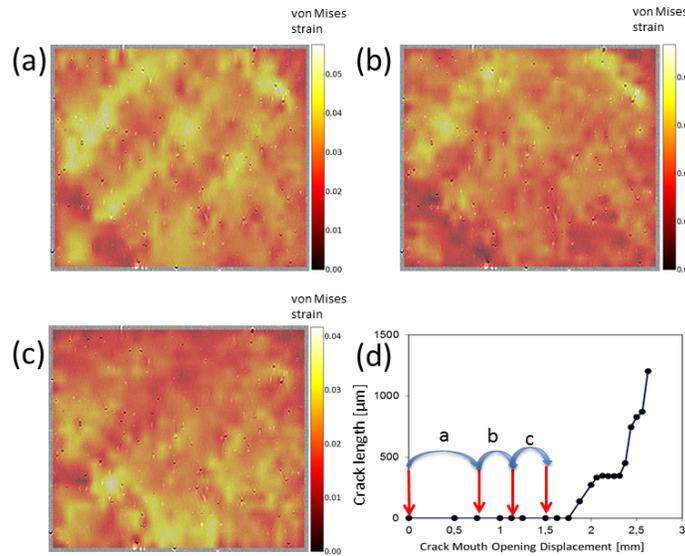
Figure 11: 2D section of 3D laminography and DVC data. Overlay of *incremental* equivalent strain fields  $n$  to  $n + 2$  (half transparent) over microstructure (the microstructure in its initial state)
