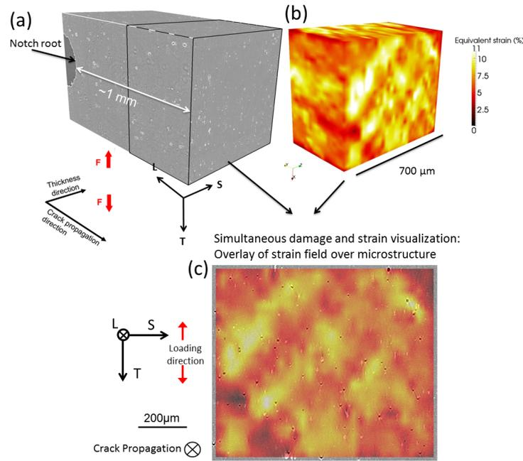
Figure 5: (a) 3D rendering of the initial microstructure and the ROI. (b) 3D rendering of the equivalent strain field in the extracted volume when  $\text{CMOD} = 1.5$  mm. (c) 2D overlay of strain field over the initial microstructure
