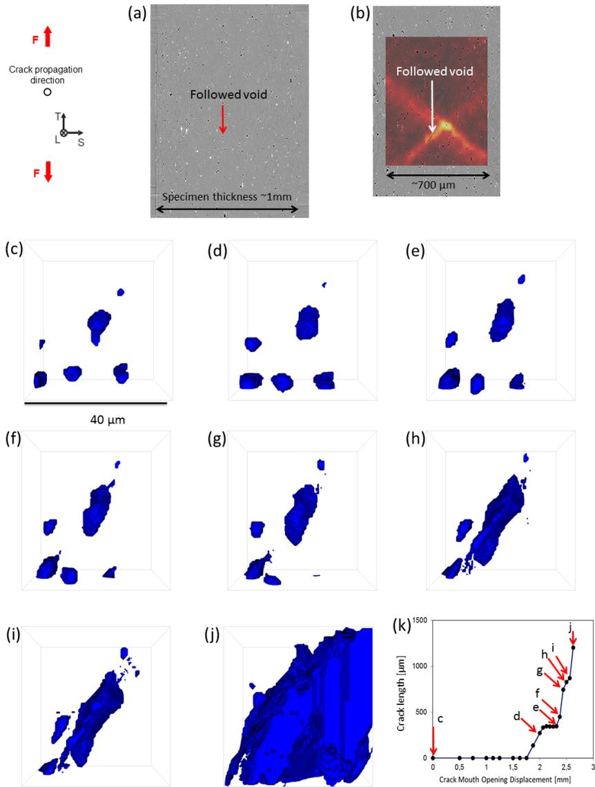
Figure 13: 3D void visualization of reconstructed laminography data. (a) Through-thickness section with location of the void  $1125 \mu\text{m}$  from the notch. (b) Overlay of strain field for step  $\text{CMOD} = 2.5 \text{ mm}$  to  $\text{CMOD} = 2.563 \text{ mm}$  over microstructure at  $\text{CMOD} = 2.5 \text{ mm}$ . (c)-(j) Void growth. (k) Indication of the corresponding load step
