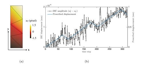
Figure 8: (a) Component  $u_Y$  of the displacement field at the last time step of the experiment evaluated via DIC. (b) Displacement amplitude  $(u_Y^+(t) - u_Y^-(t))$ in the longitudinal direction and prescribed displacement with an adapted scale (see left size of the graph)
