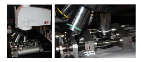
Figure 3: Experimental apparatus with the tensile stage on motorized (x,y)sample positioning stage within a Sensofar optical profiler (150× magnification lens)
