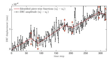
Figure 10: Displacement amplitude  $(u_Y^+(t) - u_Y^-(t))$  in the longitudinal direction from DIC (the mean of the two extreme nodes) results and the corresponding piecewise-linear steps. The arrows denote the considered degrees of freedom
