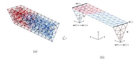
Figure 5: (a) 3D mesh of the  $\mu$ -specimen with the two grains visible (two different colors). (b) 2D mesh on the top surface used for IDIC, shown together with the sides where the boundary conditions are interpolated from the initial DIC computation
