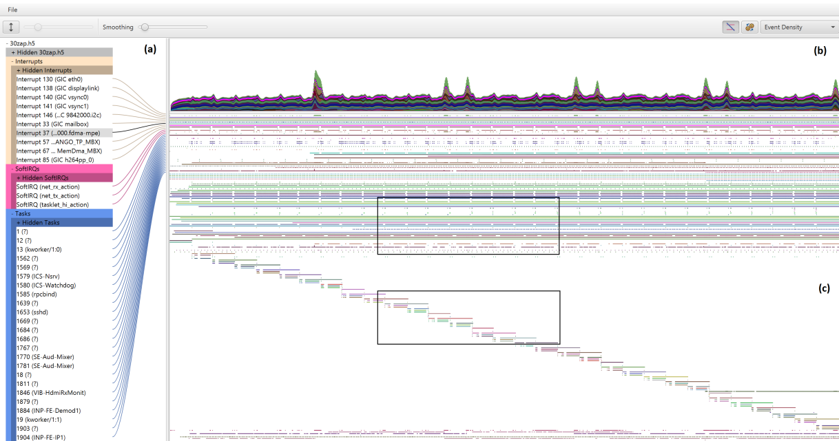
Figure 5: Overview of TraceViz. TraceViz interface consists of three main areas: the tree view (a), the outline view (b), the timeline view (c) and the links that connect the actors and their corresponding graphs (d).
