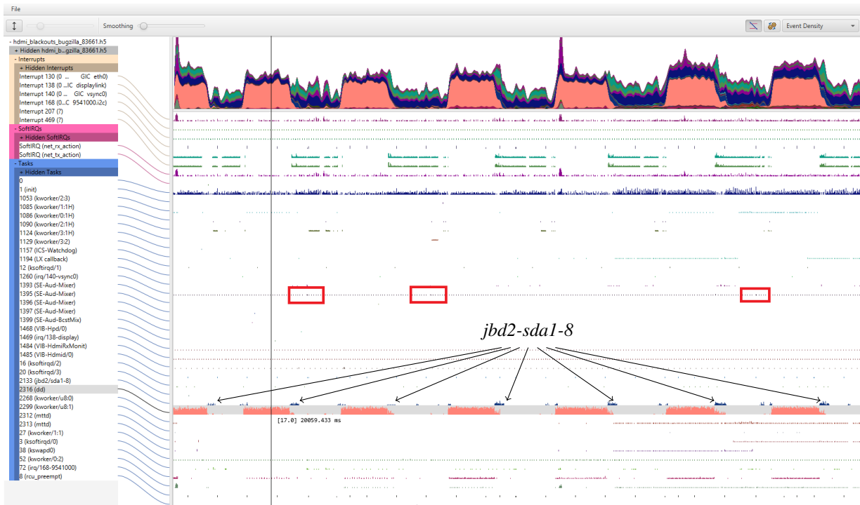
Figure 8: TraceViz showing an execution when video blanks appeared. The system is artificially loaded with heavy some I/O using the dd Unix command (in orange). The task jbd2-sda1-8 (in blue) is scheduled directly after the dd task (detailed on Figure 9), causing delays on the treatment of the VSync IRQ callback (shown in the red rectangles and zoomed on Figure 10).
