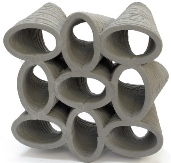
Fig. 8. Concrete 3D printed acoustic damping wall element.
