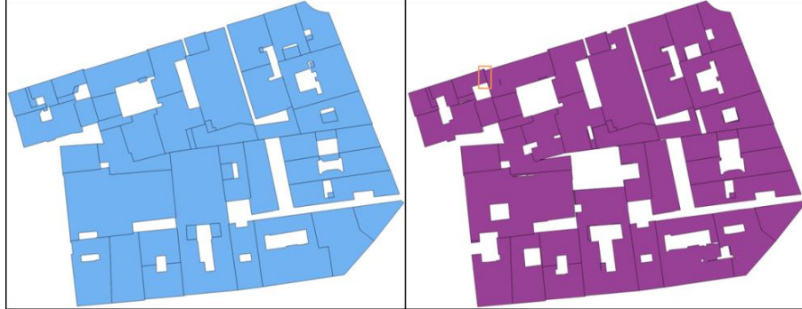
Fig. 11. On the left, cadastral polygons are extended to cover the footprint FP1 extracted from the 3D model. On the right, blue polygons are intersected with FP1 to delete the non-needed part (not present in the 3D model) and obtaining FP3 . The orange rectangle corresponds to a zoomed area used in Figure 12.
