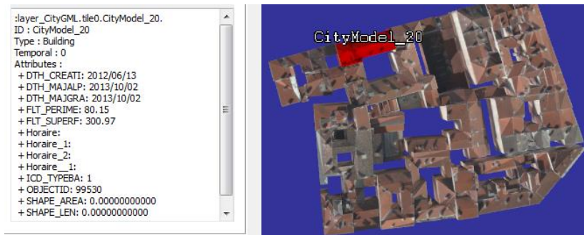
Fig. 18. Semantic information extracted from a footprint and linked to a 3D building.
