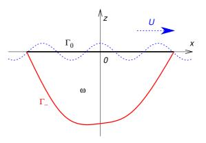
FIGURE 1. The projection  $\omega$  of the hull onto the (x, z) plane
