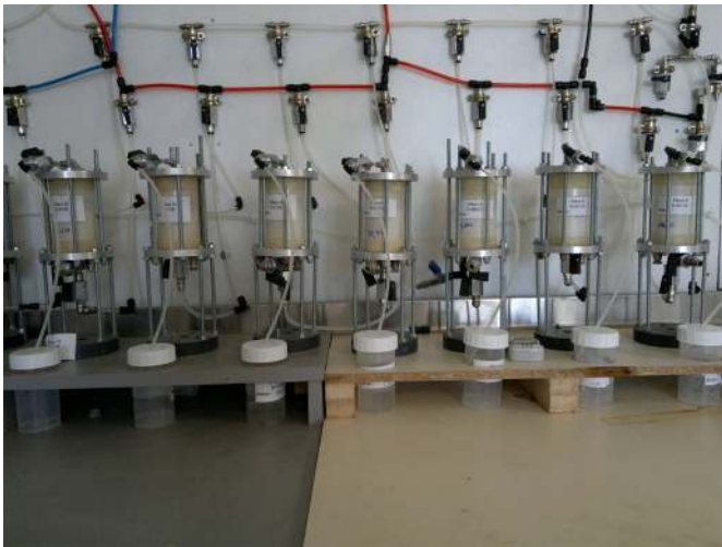
Fig. 3. Flexible-wall permeameters used for permeability tests
