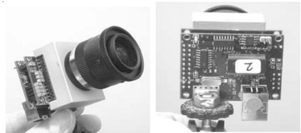
Fig. 1: Dynamic Vision Sensor (DVS) - asynchronous temporal contrast silicon retina
