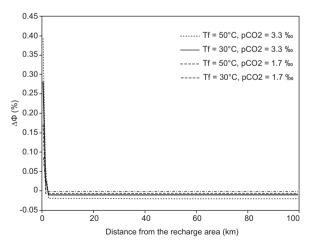
**Fig. 4.** Porosity variation  $\Delta \Phi$  along the flow line after 5 My as a function of the distance from the recharge area (x = 0), for different temperature gradients (difference between  $T_e = 20 \,^{\circ}$ C and  $T_f = 30 \,^{\circ}$ C or 50  $^{\circ}$ C), different partial pressures of CO<sub>2</sub> in the assigned input (pCO<sub>2</sub> = 1700 or 3300 ppm), and an assumed constant Darcy velocity along the flow line (U = 1 m/y).
