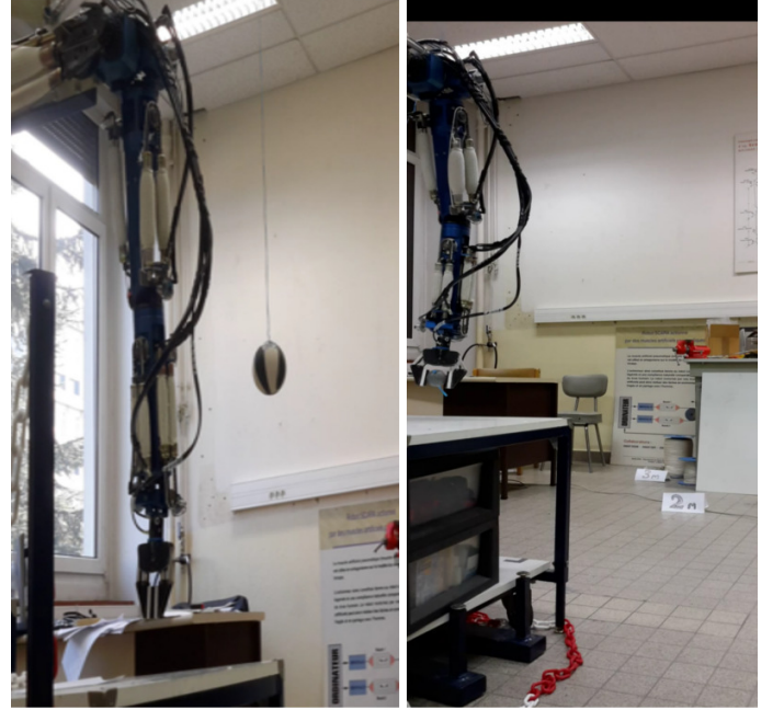
Fig. 9. Two experiments have been performed. Left picture is the set-up for the task of kicking the ball while the picture in right is the set-up for throwing the ball.
