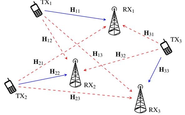
Fig. 1. A multi-user MIMO system with  $K = 3$  connections.
