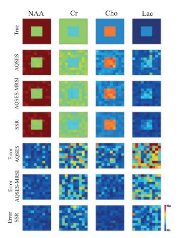
**Figure 7.** Synthetic MRSI data set containing two regions associated with healthy and tumour-like signals separated by a sharp edge. From top to bottom: true metabolite concentrations, estimated metabolite concentrations using AQSES, AQSES-MRSI and SSR and the difference (error) between the true metabolite concentrations and the concentrations estimated using AQSES, AQSES-MRSI and SSR. Errors are measured as a percentage with respect to the maximum ground-truth value for each metabolite.
