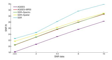
**Figure 5**. Mean SNR values computed for 50 synthetic MRSI data sets of size  $10 \times 10$  for five different noise levels (SNR values are: -0.5, 2, 4.5, 7, 10). The error bars indicate the mean RMSE<sub>k,r</sub> of the estimated metabolite amplitudes averaged over all metabolites and all voxels.
