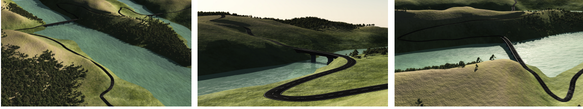
Figure 19: Different road paths obtained by modifying the relative influence of the cost functions.
