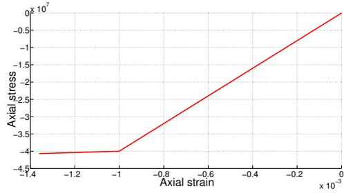
Figure 11: Behavior of the extreme compressed concrete fiber (62)
