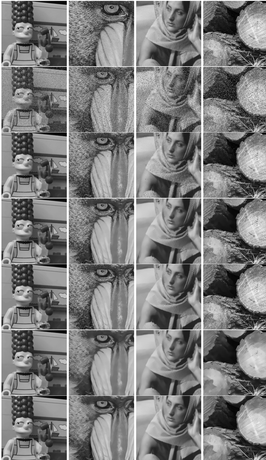
Fig. 11 Zooms of comparative results on Simpson , Baboon , Barbara and Bois with \rho = 20\% of random-valued impulse noise. From top to bottom: original images, noisy images, minimizers of E_{TV-L1} , of E_{RNL1} , of E_{RNLp} ( p = 0.5 ), of E_{NNL1} and the results of PARIGI. Images should be seen at full resolution on the electronic version of the paper.
