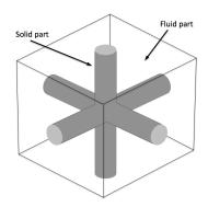
Figure 1: The unit pore Y with the solid part  $S^0$  (gray) and its complement  $Y^0 = Y \setminus S^0$ , the fluid part.
