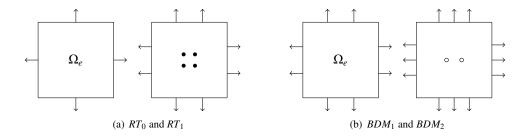
Figure 4: Degrees of freedom for two-dimensional mixed finite element spaces. Arrows indicate normal components of the velocity vector  $\mathbf{u}$  and circles represent its moments on the element interior.
