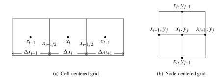
Figure 3: Examples of nodes for cell-centered and mode-centered finite differences.
