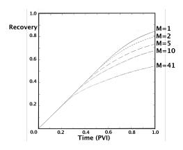
Figure 12: Example of miscible displacements with different viscosity ratios (M = 1, 2, 5, 10 and 41). Recovery curves at the production well versus time (PVI). Courtesy of Mary F. Wheeler.
