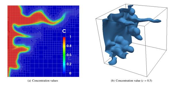
Figure 19: Two- and three-dimensional examples of unstable miscible displacements in heterogenous porous media of random permeability. For more details, see [160].
