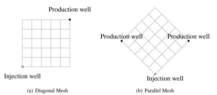
Figure 2: An example of two grid configurations in a quarter five-spot problem. Grid orientation effects may lead to vastly different computational results of flow instabilities.
