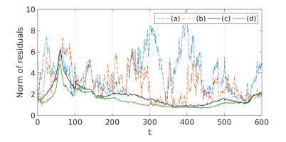
Fig. 15. Norm of the residual fields for every angles with different correction procedure: (a) average, (b) linear, (c) proposed correction, (d) proposed correction with constant absorption constraint
