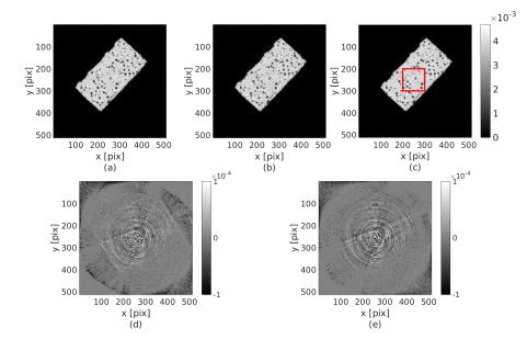
Fig. 12. Step 2. First row: SIRT reconstruction slice at z = 114 pixel normalized with (a)  $I_0^{Step}$ , (b)  $I_0^{Lin}$ , (c)  $I_0^{Prop}$ . The red rectangle shows the ROI. Second row: difference between the reconstructed slice at z = 114 pixel (d) proposed-step, (e) proposed-linear
