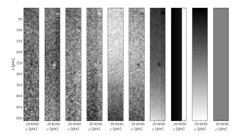
Fig. 6. Enriched flat-field library  $F_j(\rho)$  normalized with the third flat-field. The first six fields are  $F_j(\rho)$ , image 7 is the dark-field normalized with the third flat-field and the last three are added fields to help accounting for horizontal and vertical gradients and uniform intensity offset
