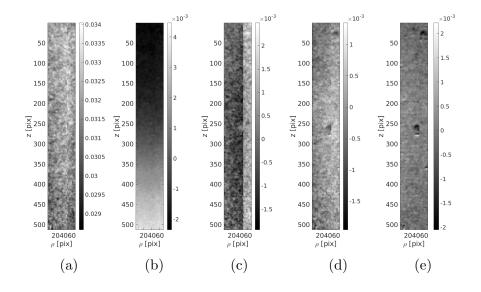
Fig. 3. From (a) to (e): spatial modes  $\Phi_n(\rho)$  for n = 1 to 5. The first spatial mode (a) has the highest eigenvalue  $\lambda_1$  and essentially represents the image intensity, (b) and (c-d) correspond to a vertical and horizontal gradient and (e) is a spot mode
