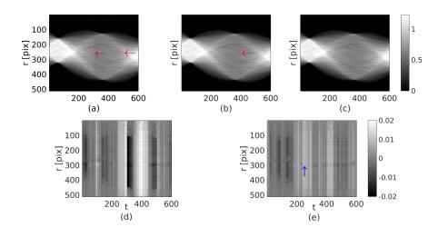
Fig. 10. Step 1. First row: sinogram (x,t) slice at z = 114 pixel corrected with (a)  $I_0^{Step}$ , (b)  $I_0^{Lin}$ , (c)  $I_0^{Prop}$ . Second row: difference between the sinogram slice at z = 114 pixel: (d) proposed – step, (e) proposed – linear. The constant absorption constraint has not been plotted because it cannot be distinguished from (c)
