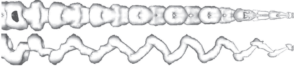
FIG. 8. Two perpendicular views of the wake structure in the zigzagging regime revealed by the \lambda_2 criterion (bubble number 19). The bubble is visible on the right.
