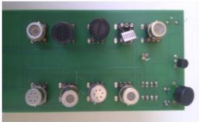
Fig 1: Sensors array including 9 semiconductor sensors
