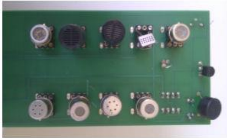
Fig 1: Sensors array including 9 semiconductor sensors
