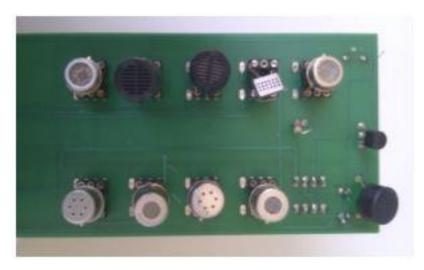
Fig 1: Sensors array including 9 semiconductor sensors
