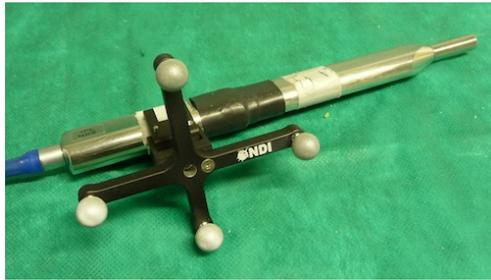
Fig. 1: (a) Beta probe and its tracking target.
