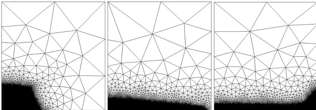
Figure 23. Adapted mesh for the dam break with shampoo at times  $t = 0.1$  (left),  $t = 0.3$  (middle) and  $t = 0.5$  (right). We see that the mesh elements' size is small inside the fluid, very small in the vicinity of the free surface and large out of the fluid far from the surface.
