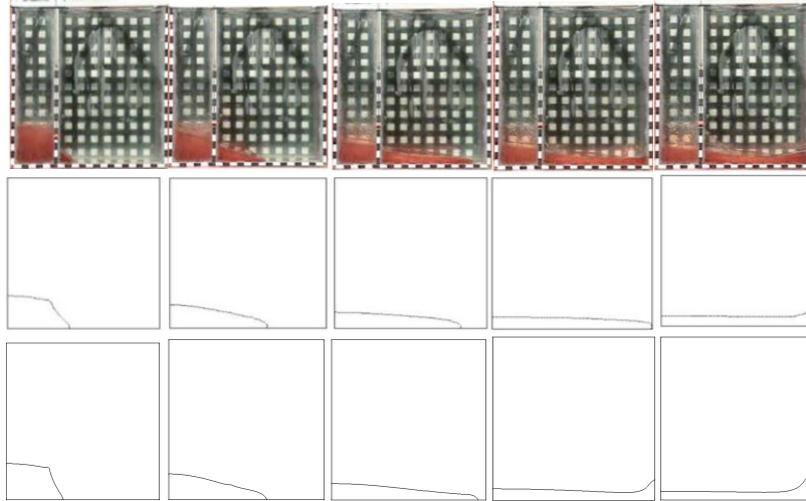
Figure 22. Comparison between physical experiments of [CCT07] (top), the numerical result of [CCT07] with wall friction (middle) and our results (bottom) at times  $t = 0.1, 0.2, 0.3, 0.4, 0.5$  (from left to right).
