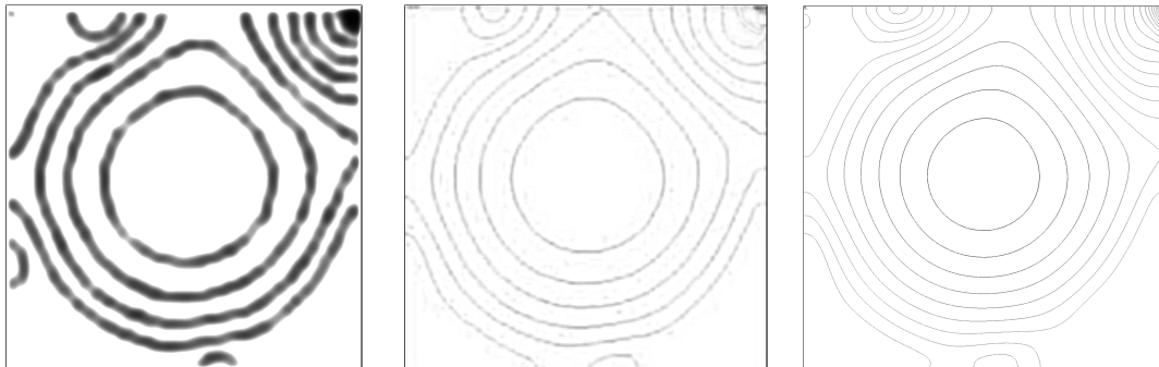
Figure 6. Cavity in 2D: Isolines of pressure with Re = 10000 . Left: result in [GWR04]. Center: result in [HRK + 10]. Right: present result
