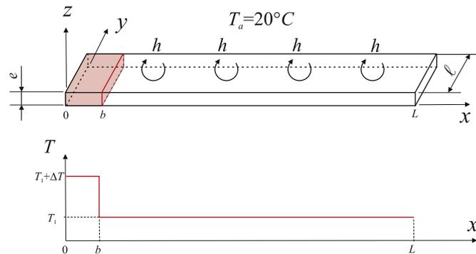
Fig. 14. Thermal model, geometry and initial conditions.
