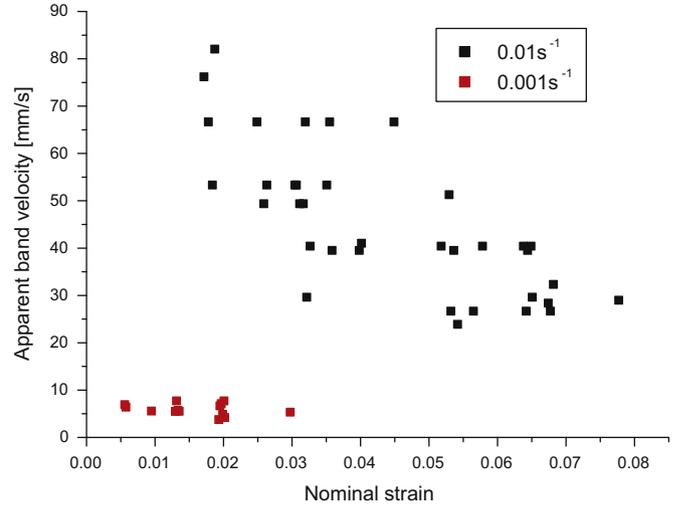
**Fig. 12.** Apparent band velocity according to nominal strain.
