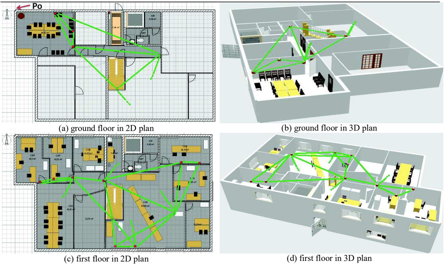
Figure 3. The 3D model of the indoor network.
