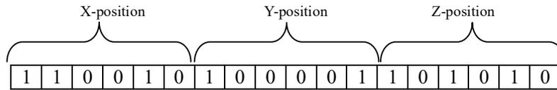
Figure1. Chromosome representing the sensor position (50, 65,42)
