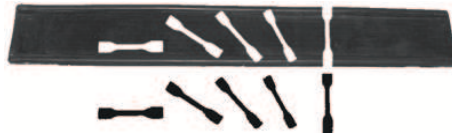
Figure 5: The pure shear sample and the secondary small dumbbells samples used for the characterisation of the anisotropic distribution of stress-softening developed under pure shear stretching
