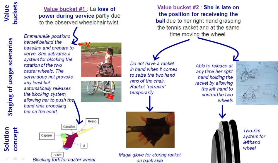
Figure 11 Illustration of the two-stage ideation process (scenario creativity and concept creativity) starting from the two value buckets identified for the handitennis wheelchair
