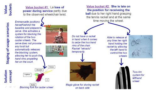
Figure 11 Illustration of the two-stage ideation process (scenario creativity and concept creativity) starting from the two value buckets identified for the handitennis wheelchair
