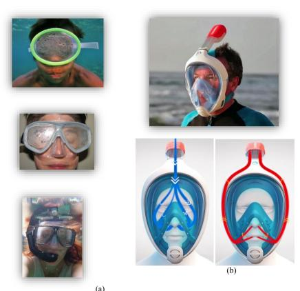
**Figure 2** Snorkeling solutions (a) Condensation and mouth breathing are common when practicing snorkeling (b) Decathlon Easybreath mask and snorkel set avoids condensation while permitting nose breathing and wide vision.
