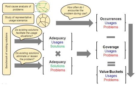
**Figure 5** The principle of the DSM Value Bucket tool for detecting and prioritizing value buckets worthwhile to further explore in creativity sessions. See also Figure 8 on the example of the handitennis wheelchair.
