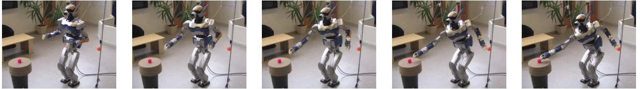
Simultaneous right-hand and left-hand reaching: the target imposed to the left hand is the final position reached in the previous (right-hand only) movement.
