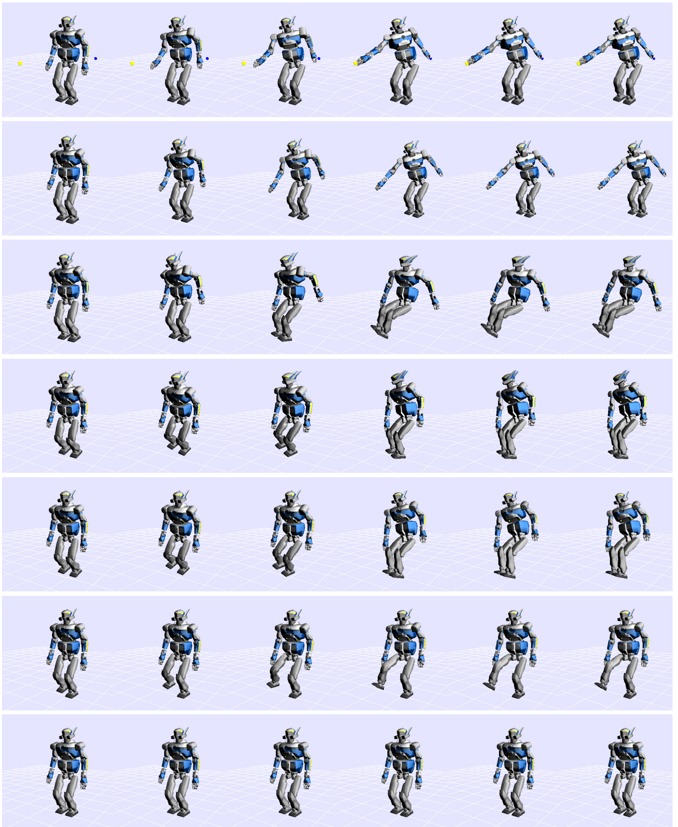
Figure 3: The original movement refers to Figure 7 (bottom): successive projection of the motion after detecting each of the seven tasks. From top to bottom: original movement; removing the right-hand task; removing the center-of-mass task; removing the gaze task; removing the left-hand task; removing the left-foot task; removing the right-foot task. On the last row, all the tasks are canceled, the projected movement is totally nullified.
