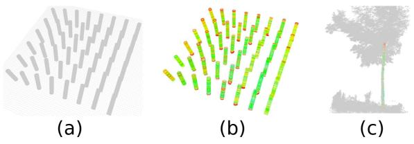
Figure 1 : (a) simulated point cloud : cylinders with increasing orientation angle and noise, (b) reconstruction with Hough transform (circles are coloured according to their value in the HS), (c) laser scanned tree stem and reconstruction as tuboid
